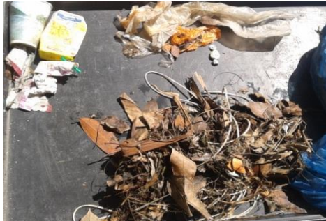
Figure 3. Sorting out gross materials more than 5mm in the CE Laboratory
